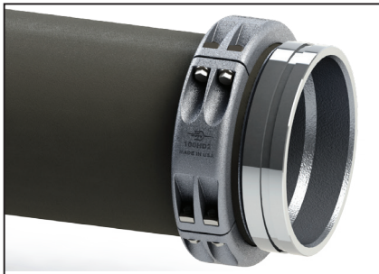
GSHD2 ASSEMBLED WITH LAY-FLAT HOSE AND HD2 CLAMP ASSEMBLY
