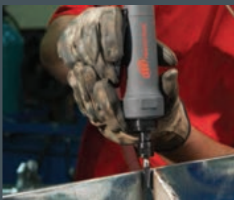
Weld cleaning and smoothing
