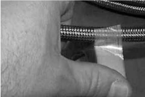
Tape hose before cutting.
