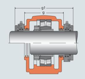
Dimensions "g" and "g1" apply to SuperTac II seals installed with FAG series SAF5..D pillow blocks. Dimensions may vary when using SuperTac II seals with non-ductile iron FAG SAF series pillow blocks, or with a non-FAG pillow block.
