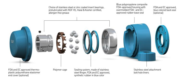
Blue Range options include a Designed For Hygiene (DFH) unit with back seal and cap, and a choice of stainless steel or zinc coating for the insert bearing. Shaft diameter range from 3/4" (20mm) - 2" (50mm).
