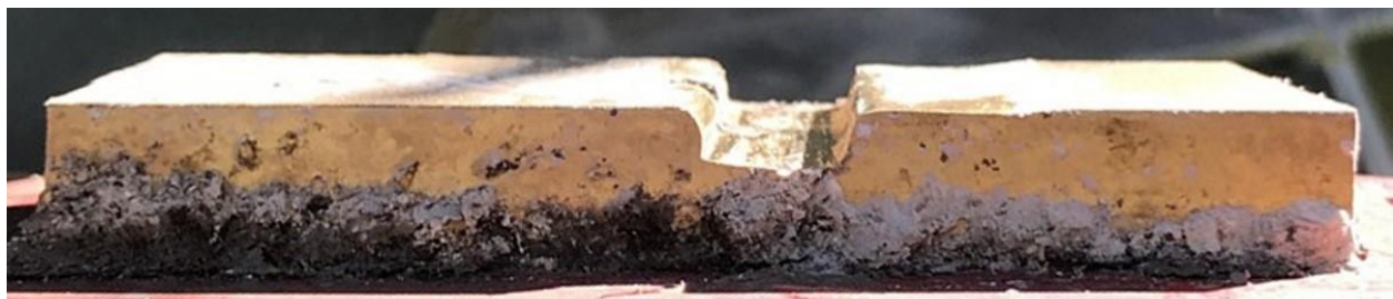
Figure 18: Brass rub block removed for inspection showing severe wear. (Photograph courtesy of 4B Components, Ltd)
